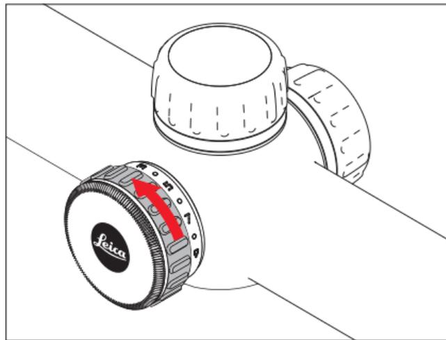
The same dial can be used to change the brightness of the illuminated dot to 9 levels to avoid any impairment when aiming with different ambient light levels:
