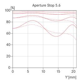
The MTF is indicated at full aperture, at f/2.8 and at f/5.6 at long taking distances (infinity). Shown is the contrast in percentage for 5, 10, 20 and 40 lp/mm accross the height of the 35 mm film format, for tangential (dotted line) and sagittal (solid line) structures, in white light. The 5 and 10 lp/mm will give an indication regarding the contrast ratio for large object structures. The 20 and 40 lp/mm records the resolution of finer and finest object structures.
