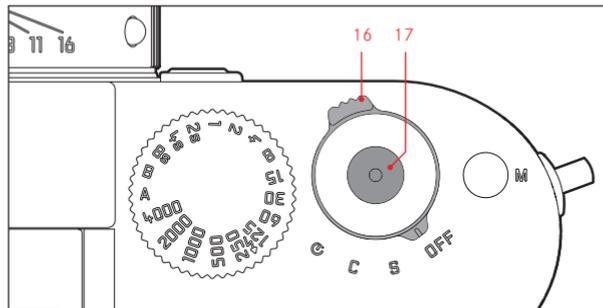
The camera is turned on and off using the main switch (16). This is below the shutter release (17) and is a lever with four detent positions:
