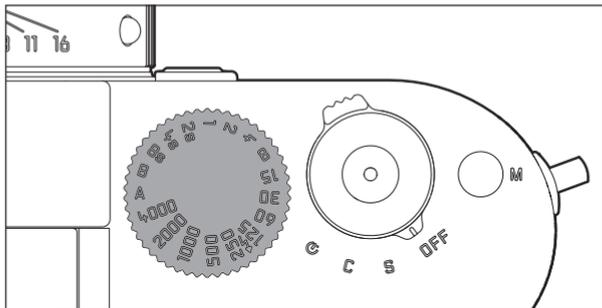
The exposure modes are selected using the shutter speed dial (19),
