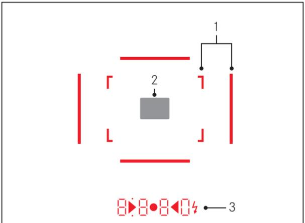
1. Bright line frame for 50mm and 75mm<sup>1</sup> (example)
